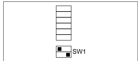
Figure 18: SW1 setting for current measurement by internal summation of phase currents
