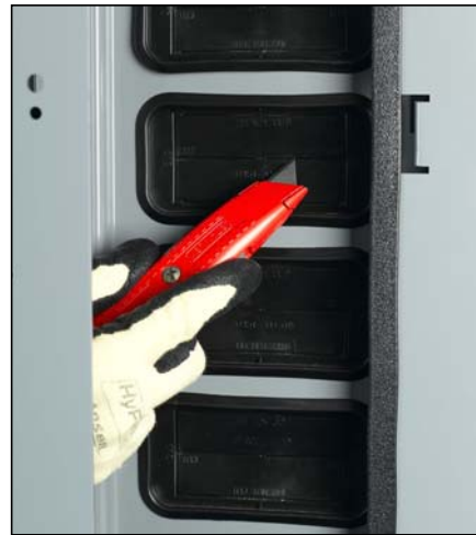
Figure 62: Vertical Wire Trough Grommet
