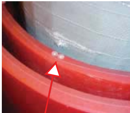
Figure 4B: Thermowell Hole
