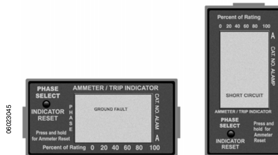
Figure 14. Trip Condition Displays on ALAM and ALAMP Ammeter/Trip Indicators
