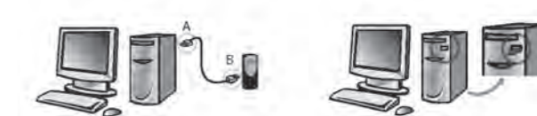
A: USB type A connector B: USB Mini-B type connector
