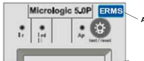
Figure 1: ERMS Label on Trip Unit
