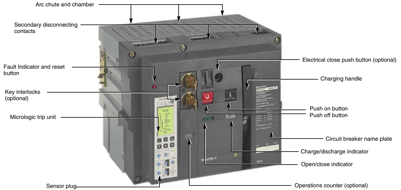
Figure 16: Masterpact NW Circuit Breaker (Front and Side View)
