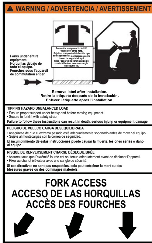
Figure 4 – Rear Warning Label, Rainproof Switchboards
