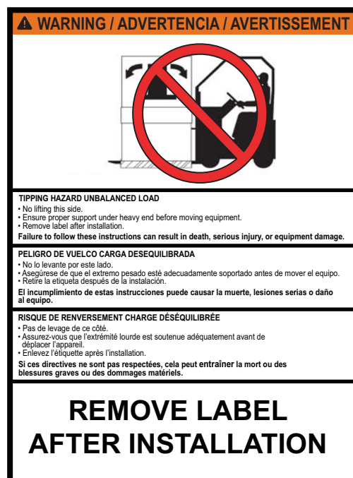
Figure 5 – Front Warning Label, Rainproof Switchboards
