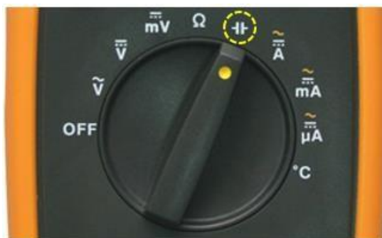
Figure 15-Setting DMM to measure Capacitance
