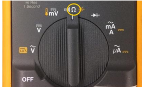
Figure 14- Setting DMM to measure Ohms
