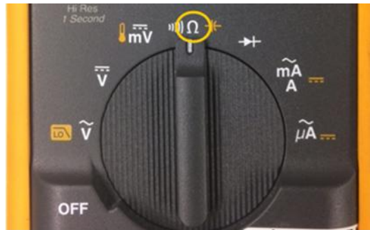
Figure 10-Setting a DMM to measure ohms
