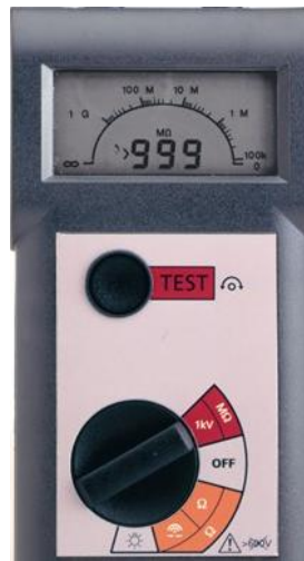
Figure 12-Megger insulation resistance meter
