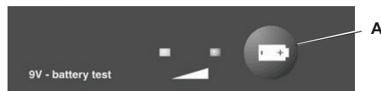
Figure 13: Battery Test Button
