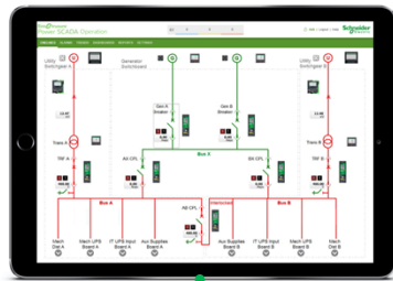
Power SCADA Client
