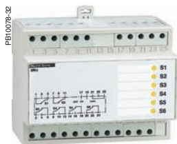
M6C programmable contacts: circuit-breaker external relay with six independent changeover contacts controlled from the circuit breaker via a three-wire connection.
