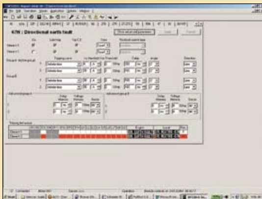
Directional Ground Overcurrent Protection
