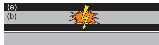
Figure 1 - (a) Metal layer - (b) Polypropylene film
