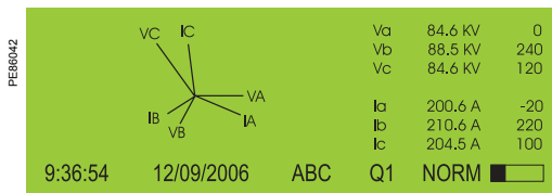
ION8650 front panel phasor display and table.
