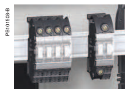
Possibility to transform the terminal block into an incoming splitter block up to 125 A, thanks to the support PRA90048.
