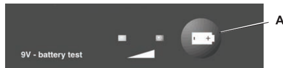
Figure 13: Battery Test Button
