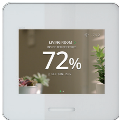
Figure 19. The Wiser Home Touch acts as the central transmission device in your Wiser network. It connects your smartphone to your Wiser devices via your router. In this system, your smartphone and Home Touch will communicate via Wi-Fi.
