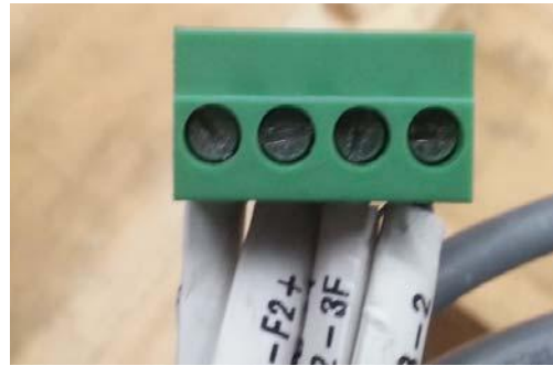
Figure 41: Example of Modbus RS485 4-pin Plug
