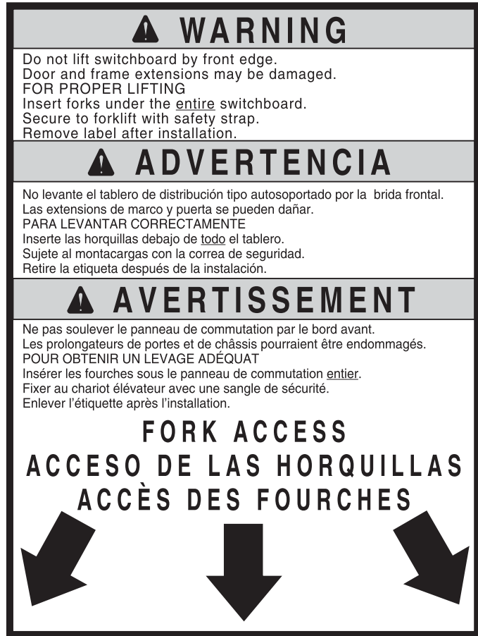
Figure 4: Warning Label, Rainproof Switchboards
