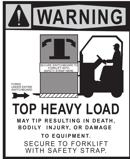
Figure 7: Forklift Safety Strap
