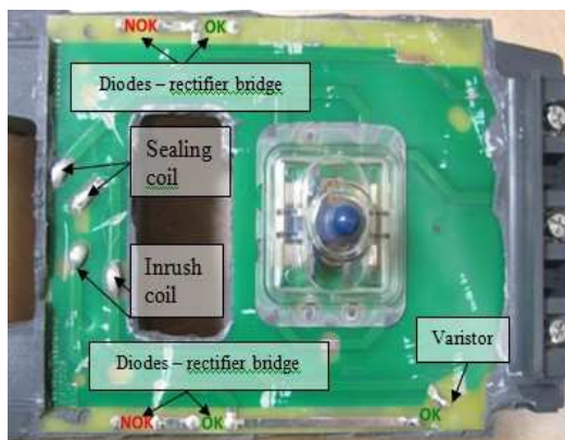
6 - PCB card after removing over molding material
