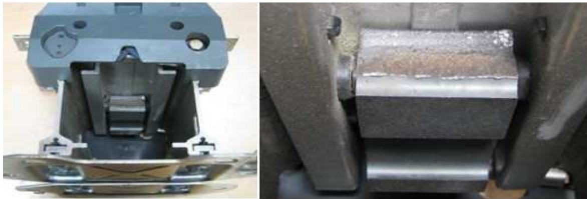
6 – Damaged mobile magnet.
