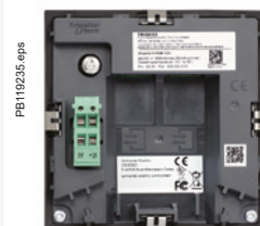
Connection with FDM121 display unit.
