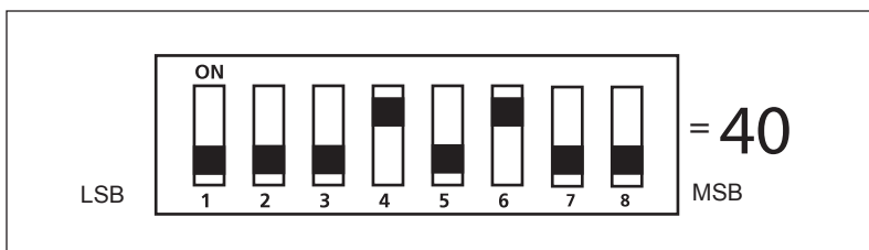
Figure 18 Modbus® address DIP switch values
