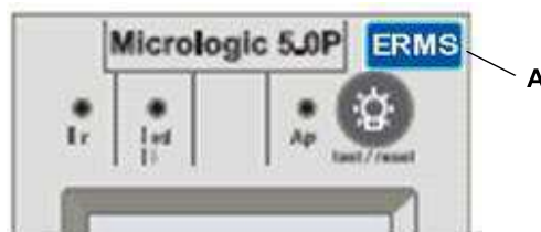
Figure 1 – ERMS Label on Trip Unit
